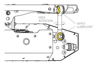
Do not, under any circumstances, allow the lubricant to get inside the motion platform from section because it might contaminate reference position sensor and affect the start-up calibration routine. If the worse case scenario, the motion platform will not be able to calibrated correctly and it will stop working until sensors are cleaned or replaced.
